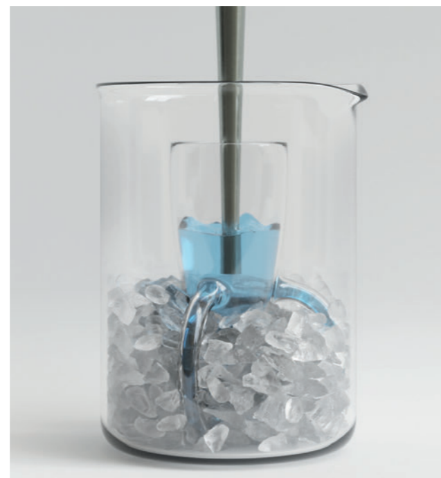
Cooling the sample in a rosette cell RZ with crushed ice
