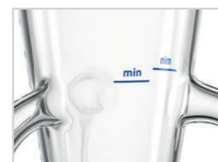
Marking of the minimum fill level
