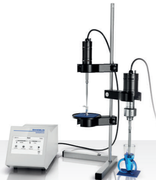
Sonication of two samples on one stand
